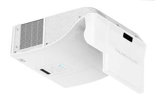
Multi touch technology integrated directly into the projector – no extra interactive whiteboard needed. The Laser Curtain module easily mounted onto the standard flat board creates an IR beam that covers all the board. The IR camera integrated with the projector senses a finger, stylus or pen touch onto the surface, up to 10 touch points simultaneously!
