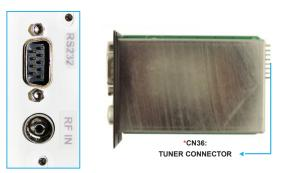
TRIUMPH BOARD TV TUNER T1 for MULTI Touch LED LCD provides a wide range of connectivity to Analog and Digital TV signal across the Europe, Middle East, Russia, North and South Africa. Device also comes with the additional RS232 port for the extended possibility of remote control of your TRIUMPH BOARD MULTI Touch LED LCD.
