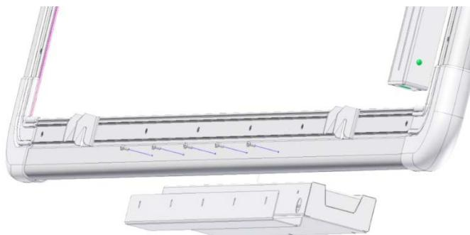
If you have an older model of the TRIUMPH BOARD RESISTIVE it may be that there are no pre-drilled holes on the lower rear frame. In this case please drill the 2.5mm holes into the frame that will align with the pre-drilled holes on the Pen Tray, and then install the Pen Tray as described above.
