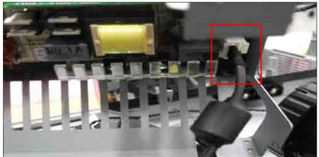
3. Unscrew 1 screw (as green circle) to disassemble the thermal sensor board.
