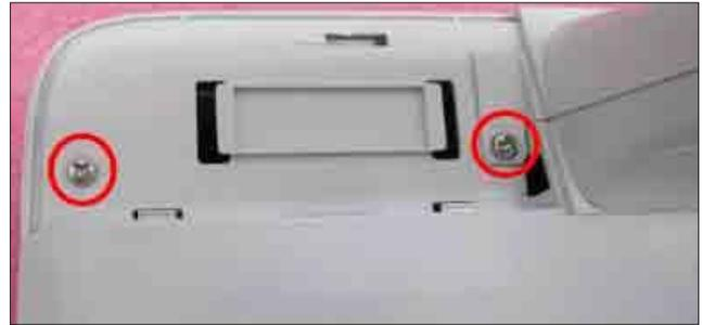
2. Disassemble the Bottom Cap (as green square).
