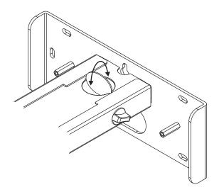
i. Insert Cable Protection Grommet and feed Cables in to support.
