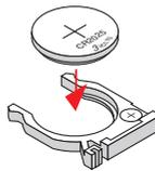
Remove the old battery and install new one (CR2025). Ensure that the side with a "+" is facing up.
