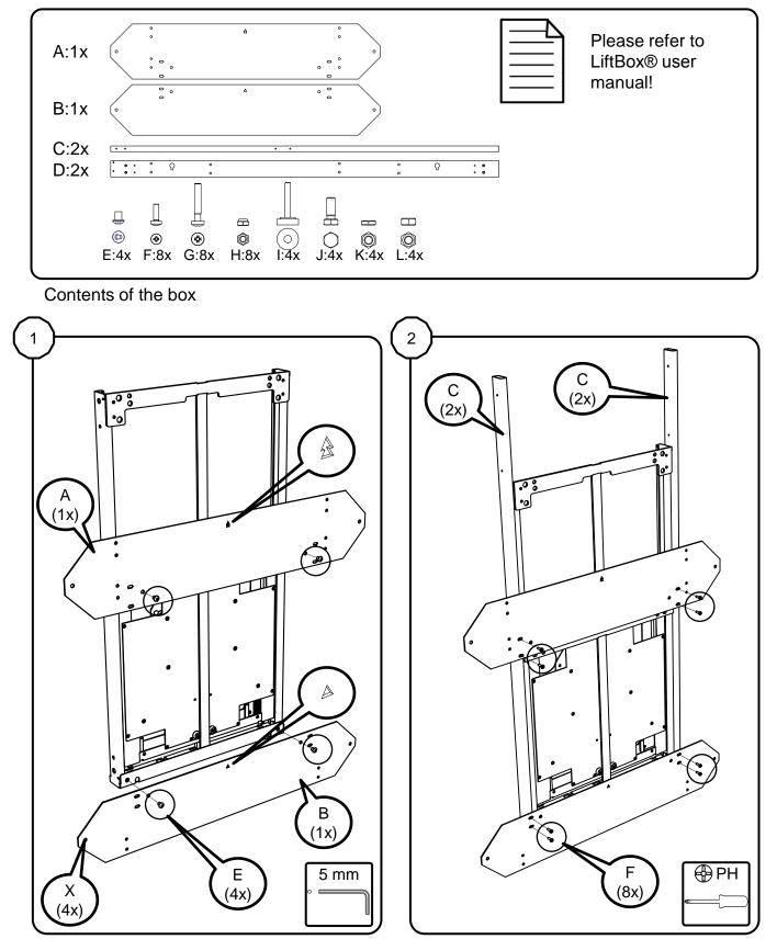
Mount top and bottom base plates to LiftBox<sup>®</sup> (not included) (Holes X for mounting on LiftBox 650)
