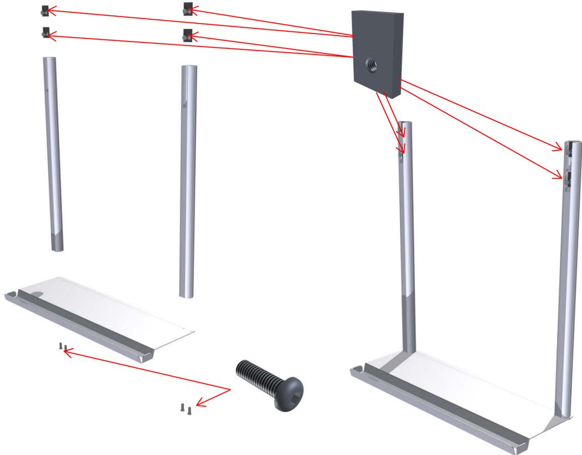
Insert the 2 aluminum rods through the inside of the cabinet of TRIUMPH BOARD Mobile Stand with Electric Lift for LED LCD's.
