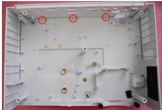
3. Separate bottom cover module and IO cover.
