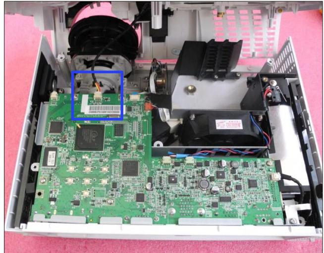
5. Disassemble the top cover module.
