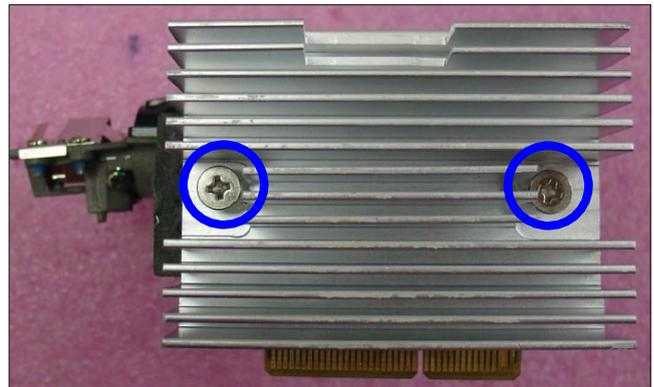
6. Disassemble the heat sink and DMD module, and then tear off 2 DMD molars (as green square).
