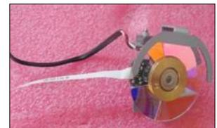
3. Unscrew 1 screw (as blue circle) to disassemble the photo sensor board.
