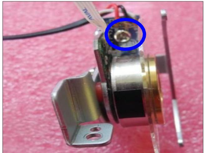
4. Separate the photo sensor board and spacer.
