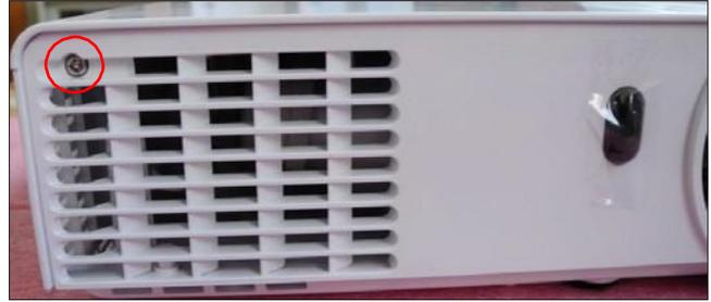
2. Loosen 2 screws (as yellow circle) on the lamp module.
