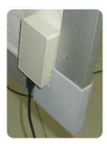
For the interactive whiteboard connection, one USB cable is needed. There is no extra power supply required for this product. After connecting the cable between the USB interface of PC and the interface of the interactive whiteboard, the connection is completed. After successful installation, the indicator of the interactive whiteboard becomes green.
