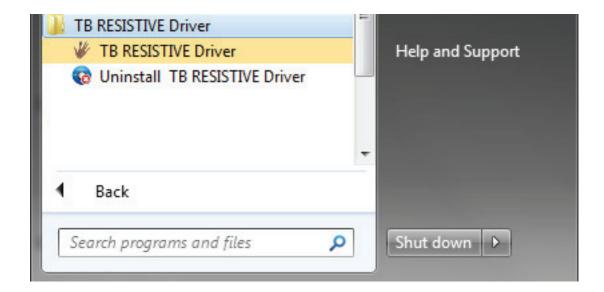
Please Note: You need to re-adjust when the following situations: Move the TRIUMPH BOARD RESISTIVE interactive whiteboard; Move the projector; Re-install TRIUMPH BOARD Drivers; Change the computer resolution.
