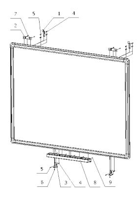
Install suspender (2) with screws(7) to the board.
